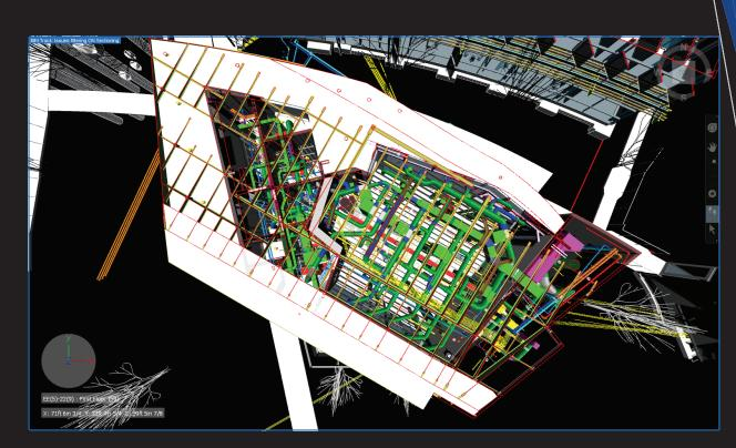
The mechanical, electrical, and plumbing (MEP) coordination efforts through Building Information Modeling (BIM) are wrapping up this month. The model will then be used to verify work in the field.
